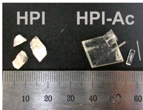
Figure 1. Photograph showing single crystals of HPI and HPI-Ac (ruler scale is in millimeter units).
